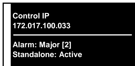
Figure 3.3 Viewing Alarms on the Front Panel
