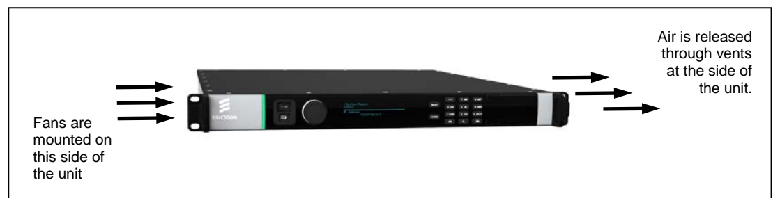
Figure 2.1 Air-Flow through the Equipment
