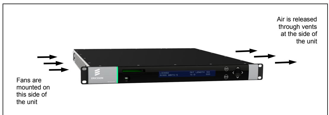
Figure 2.1 Air-flow through the Equipment
