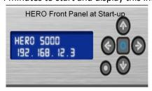
3. From your workstation located on the same subnet, open a web browser and enter the IP address assigned to the HERO into the address bar.
