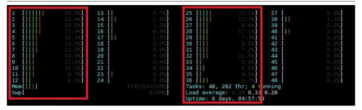
Here we can see that with a single service, all of the work is being done by one NUMA node, the activity on the other NUMA node is just basic OS tasks.
