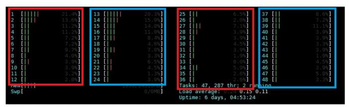
The two red boxes are for the first NUMA node, the blue boxes are for the second NUMA node. In the above example we can see that although the MFEL is only running a single service, some cores from each NUMA node are being used.
