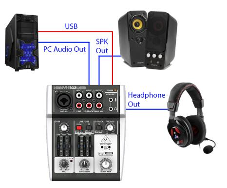
The USB Mixer is connected to the PC via USB, the USB supplies Power, and the Mixer is also a Windows USB Audio Device (so works as a soundcard in it's own right).
