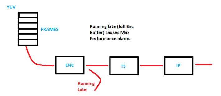
Looking at the above diagram, if for some reason there is an issue with the output of the MFEL, and if there are no Running Late alarms, then the output issue is not related to the encode process (probably) rather another mechanism within the MFEL.
