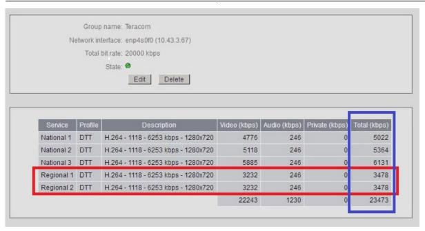
Here we can see that the Stat Mux pool (at the top of the image) is 20000 kbps and that Regional 1 and Regional 2 (in the red box) are both the same bit rate (at this instance in time).
