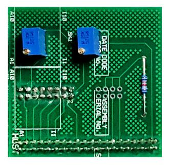
The Driver Board has two Potentiometers (10K or 20K are fine) for adjusting backlight and LCD contrast. The 40 Way header for connecting to the Raspberry Pi and a 16 Way ribbon cable that goes to the LCD.
