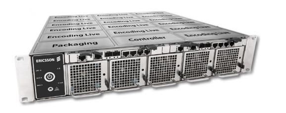
The T1 is a new platform based on a server that can have up to 9 Blades fitted. Each blade contains two separate servers. The T1 main differentiator (at launch) is that it is the first platform that can take advantage of the QSV (Quick Sync Video) feature of the Intel Processor.
