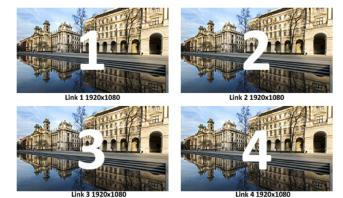
2SI method allows picture monitoring on standard 1080P displays as each link carries the whole image at 1/4 of its original resolution
