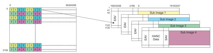
The interleaving is done two samples at a time, so from the top left quadrant (1) and the top right quadrant (2) we order the pixels 2×2. Hence the 112211221122 pattern. The same is also performed on quadrants 3 and 4. The two pixel interleave is alternated down the frame on each line.
