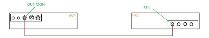
The Monitor F-Type output of the AVP is connected directly to the RF input of the RX1 (RX4 is on the left). There is no up-convertor or attenuator in use.
