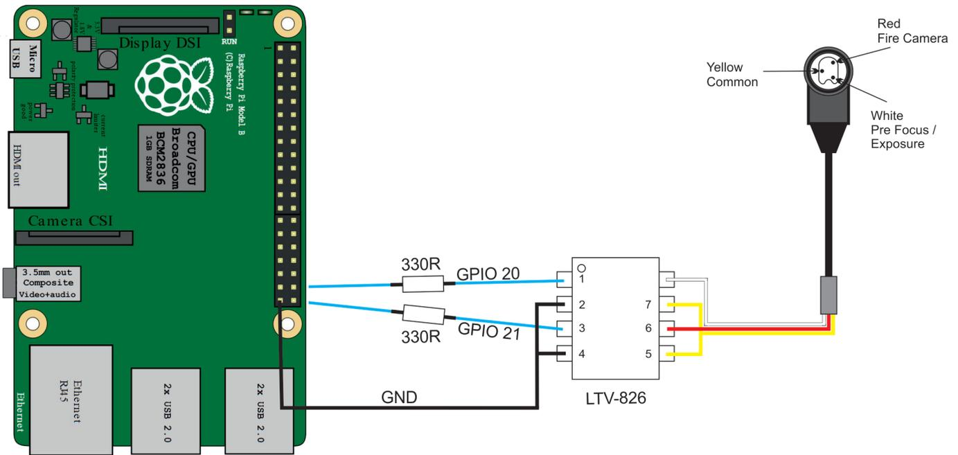
**WARNING!!!** - The left and right parts of the circuit are independent. Do not connect the common connection on the right to the GND on the left.
