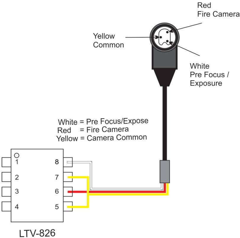
Here we can see a close up of the plug and circuit, I have used Red, White and Yellow wires because I purchased a cheap shutter release cord for my camera, and cut off the button, and these were the wiring colours. Are they standard? don't know.
