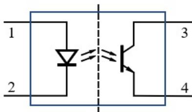
We use a resistor between the output of the GPIO Pin (3.3v remember) to limit the current to the input diode (pin 1 on the Opto-Coupler), this drives the output on pin 4. We use the output pins (3 & 4) like a switch, shorting what is on pin 3 to pin 4 when the input on pin one goes high.
