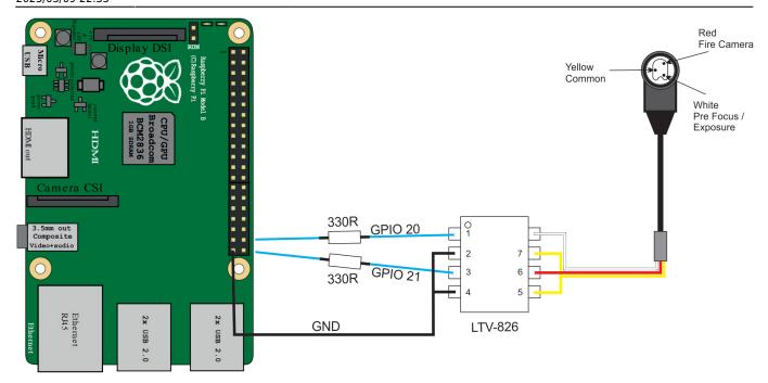
WARNING!!! - The left and right parts of the circuit are independent. Do not connect the common connection on the right to the GND on the left.
