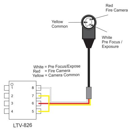
Here we can see a close up of the plug and circuit, I have used Red, White and Yellow wires because I purchased a cheap shutter release cord for my camera, and cut off the button, and these were the wiring colours. Are they standard? don't know.
