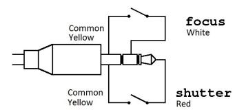
The circuitry is identical, it's just the connector type that changes.
