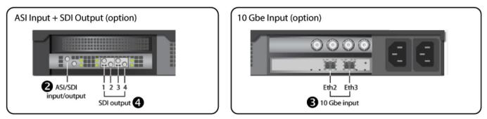
The four normal BNC connectors top right are for ASI Inputs.
