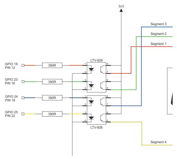
You can think of these as an electrical switch, operated by light. On the left hand side of the device, you supply a small current via a resistor (that is connected to a GPIO pin) and this turns on the LED in the package, this allows a current to flow on the right hand side, this current can be much greater than the input current. This stops too much current being pulled from the Raspberry Pi.
