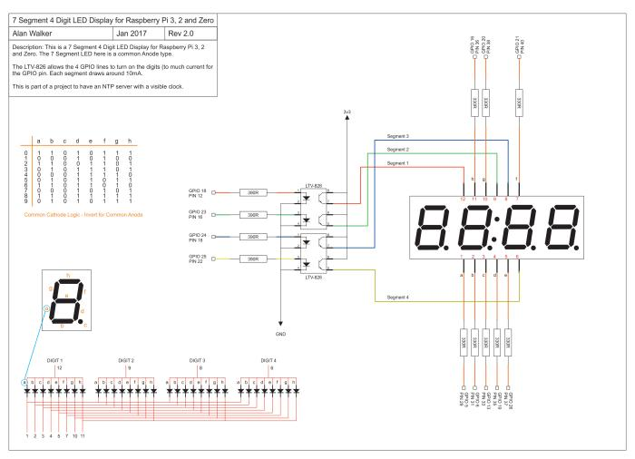
There are two Opto-Isolators to control the four digit lines. These are required because the Pi can't supply enough current (a whole 7 Segment digit using all segments requires around 40-50 mA, a GPIO pin should only sink or source around 16 mA).
