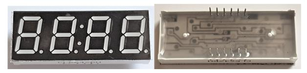
Common Anode vs Common Cathode - All LEDs have a positive (Anode) and negative (Cathode) connection. On a common Anode display, all
