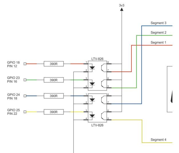
You can think of these as an electrical switch, operated by light. On the left hand side of the device, you supply a small current via a resistor (that is connected to a GPIO pin) and this turns on the LED in the package, this allows a current to flow on the right hand side, this current can be much greater than the input current. This stops too much current being pulled from the Raspberry Pi.
