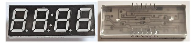
Common Anode vs Common Cathode - All LEDs have a positive (Anode) and negative (Cathode) connection. On a common Anode display, all
