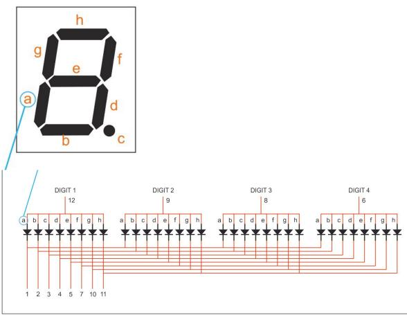
Above is the connections for my 7 Segment LED Display. Mine has 12 pins. Four pins for the selection of the Digit (which number is on) and 8 pins for the individual segments. There are 8 pins because this display has a full stop after each digit.
