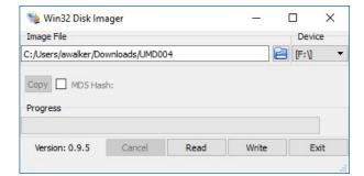
When downloading a Linux Distribution, just remember to download the ISO (rather than installer) and use Win32 Disk Imager to write the ISO to either your Micro SD Card or USB Device.
