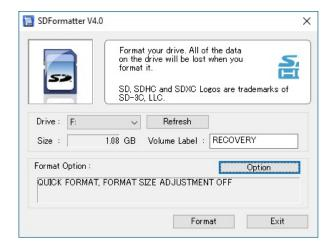
Most Linux distributions will create an array of partitions on your Micro SD Card, and the easiest way to get rid of all of them, so you can start a fresh install is to use the SDFormatter application. SDFormatter works with USB sticks as well.
