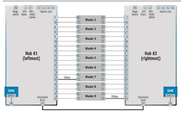
On the Rear of the T1 chassis we can see the blades and Servers (each Blade has two Servers) to ensure you are connecting to the correct one, please refer to the diagram below:
