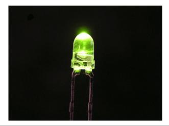
Turning on LEDs using the GPIO on the Raspberry Pi is pretty simple. You just turn on or off the relevant GPIO pin, and your LED (connected via a 330r resistor) will come on and go off.
