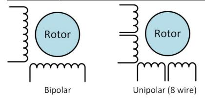
**Unipolar drivers** always energize the phases in the same way. One lead, the "common" lead, will always be negative. The other lead will always be positive. Unipolar drivers can be implemented with simple transistor circuitry. The disadvantage is that there is less available torque because only half of the coils can be energized at a time.
