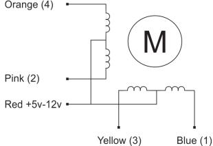
The coils have to be activated in the correct order, or you will find that the stepper motor is slow, has little torque, won't move at all or just gets really hot.
