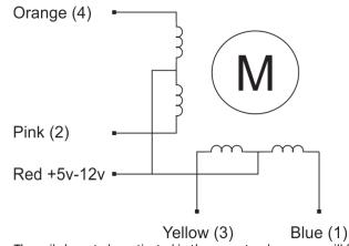
The coils have to be activated in the correct order, or you will find that the stepper motor is slow, has little torque, won't move at all or just gets really hot.
