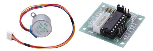
This is the five wire type mentioned above. The Stepper motor comes with a little driver board, normally ULN2003 based, this board has four LEDs so you can see the drive lines go high and low, very handy for troubleshooting.
