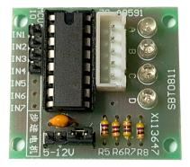
The IN1-IN4 are the connections to the Raspberry Pi GPIO Pins. There is a Gnd and +Ve connection below the INx Pins. The white connector is for the Stepper Motor header, and the four LEDs show you which IN1-IN4 phases are present at any one time (under normal operation these flash so fast they all look they are on, but you can slow this down).
