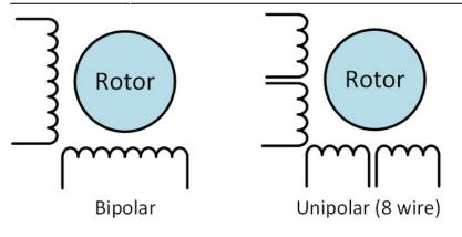
**Unipolar drivers** always energize the phases in the same way. One lead, the "common" lead, will always be negative. The other lead will always be positive. Unipolar drivers can be implemented with simple transistor circuitry. The disadvantage is that there is less available torque because only half of the coils can be energized at a time.
