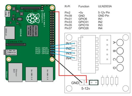
Yep, six wires is all we need. If you are using the same stepper motor as in this example (the 28BYJ-48) then the total current draw of your Pi will be around 500mA (depending on what you have plugged in). This is will within the 1Amp you can get out of the 5V supply.
