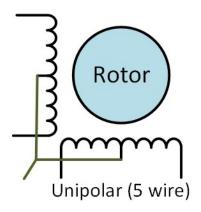
This style is common in smaller unipolar motors. All of the common coil wires are tied together internally abd brought out as a 5th wire. This motor can only be driven as a unipolar motor. This is the type of Stepper Motor that I am using in this example.
