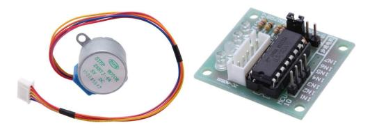
This is the five wire type mentioned above. The Stepper motor comes with a little driver board, normally ULN2003 based, this board has four LEDs so you can see the drive lines go high and low, very handy for troubleshooting.
