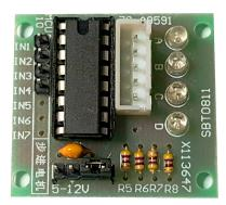
The IN1-IN4 are the connections to the Raspberry Pi GPIO Pins. There is a Gnd and +Ve connection below the INx Pins. The white connector is for the Stepper Motor header, and the four LEDs show you which IN1-IN4 phases are present at any one time (under normal operation these flash so fast they all look they are on, but you can slow this down).
