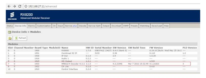
For existing RX8200s there is an option for them to decode HEVC, depending on what option cards are fitted. Firstly there has to be a 4:2:2 decoder card, and this card has to be one of the following types:
