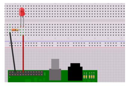
This is a red LED that has a 2V drop across it, so 3.3v-2v = 1.3v. The LED only needs around 5mA, so R=V/I = 1.3/0.005 = 260 Ohms.
