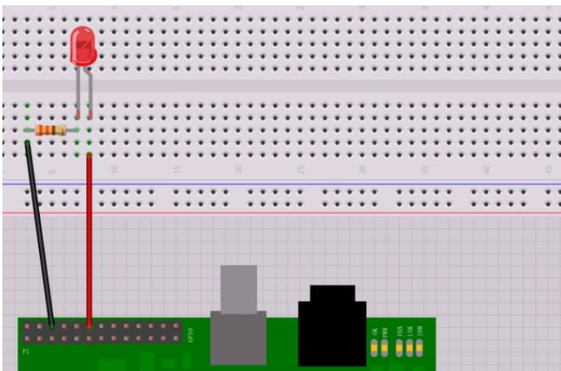
This is a red LED that has a 2V drop across it, so  $3.3\text{v} - 2\text{v} = 1.3\text{v}$ . The LED only needs around 5mA, so  $R = V/I = 1.3/0.005 = 260$  Ohms.
