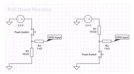
So for any input that we are waiting for a high signal (3.3v) we will use pull down so it stays a 0v, for any pin we are waiting for a low signal (0v) we will use a pull up so it stays at 3.3v (until a button press makes it low)
