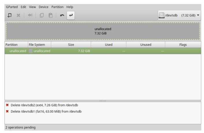
Once all of the partitions are removed, we have to click the arrow at the top of the gparted interface to accept the changes (just under the word Help in the above image).
