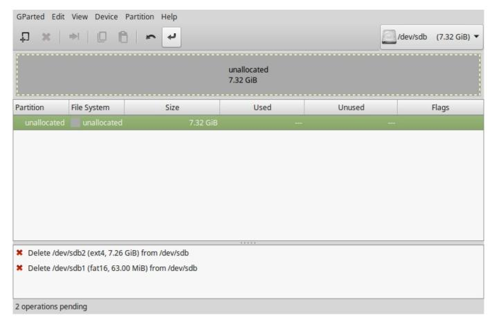
Once all of the partitions are removed, we have to click the arrow at the top of the gparted interface to accept the changes (just under the word Help in the above image).
