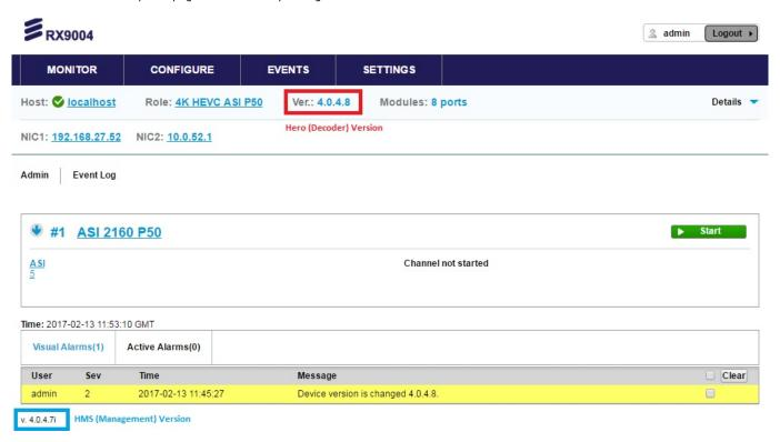
The version in the top centre of the page is the HERO (Decoder) version, and the bottom left is the HMS (Management System) version.
