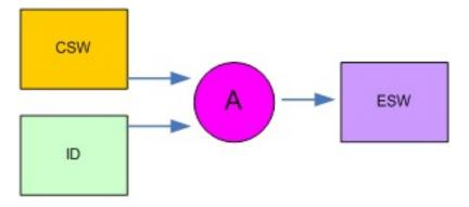
When generating BISS-E keys for distribution to clients, you will know the CSW and the ID for each receiver. A software application then generates the ESW.
