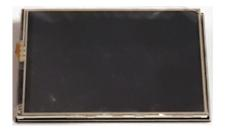
At around £8, adding a full function LCD display to a Raspberry Pi that is running without any attached monitor is a great way to add a bit of simple monitoring, or if required a more complex control system for stand alone projects.
