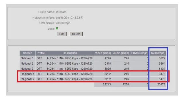
Here we can see that the Stat Mux pool (at the top of the image) is 20000 kbps and that Regional 1 and Regional 2 (in the red box) are both the same bit rate (at this instance in time).
