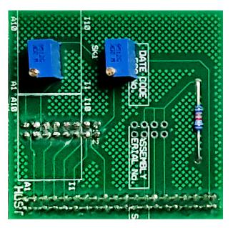
The Driver Board has two Potentiometers (10K or 20K are fine) for adjusting backlight and LCD contrast. The 40 Way header for connecting to the Raspberry Pi and a 16 Way ribbon cable that goes to the LCD.
