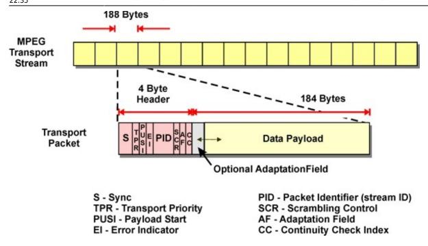
In the above diagram it can be seen that the overall format of the TS packet is as follows:
