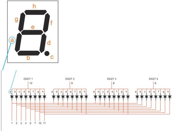
Above is the connections for my 7 Segment LED Display. Mine has 12 pins. Four pins for the selection of the Digit (which number is on) and 8 pins for the individual segments. There are 8 pins because this display has a full stop after each digit.
