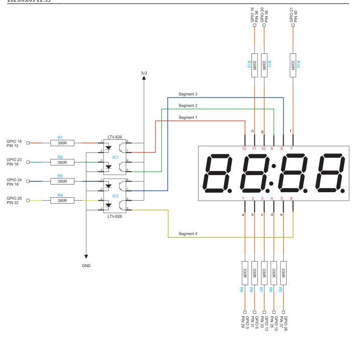
There are two Opto-Isolators to control the four digit lines. These are required because the Pi can't supply enough current (a whole 7 Segment digit using all segments requires around 40-50 mA, a GPIO pin should only sink or source around 16 mA).
