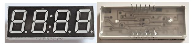
Common Anode vs Common Cathode - All LEDs have a positive (Anode) and negative (Cathode) connection. On a common Anode display, all the Anodes (positives) are joined together, so you can only control the negative side of the LED segments. This means you switch each segment on by connecting or disconnecting the negative pins.
