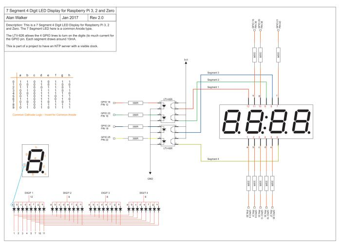
There are two Opto-Isolators to control the four digit lines. These are required because the Pi can't supply enough current (a whole 7 Segment digit using all segments requires around 40-50 mA, a GPIO pin should only sink or source around 16 mA).
