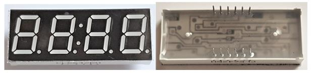
Common Anode vs Common Cathode - All LEDs have a positive (Anode) and negative (Cathode) connection. On a common Anode display, all
