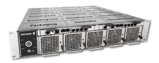
The T1 is a new platform based on a server that can have up to 9 Blades fitted. Each blade contains two separate servers. The T1 main differentiator (at launch) is that it is the first platform that can take advantage of the QSV (Quick Sync Video) feature of the Intel Processor.
