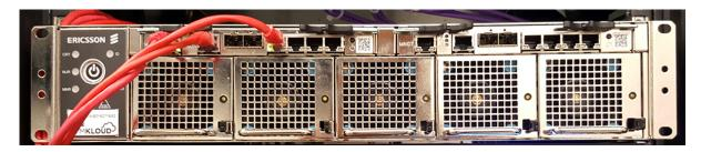
The front of the T1 Chassis has five removable fans (hot swap), the power button and access to the two switches. The unit does automatically power up when the power cables are inserted. The power cables are the type that have a notch in them, so standard IEC cables will not fit.
