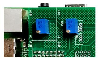
Adjusting these two potentiometers will allow you to balance the text and backlight intensity to get the brightness level you require.
