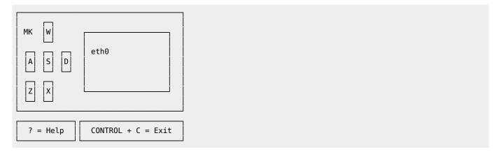
To get the NTP settings, you have to scroll down using 'X', however, it depends on how many physical interfaces the RX1 has that dictates how many times you have to scroll down.
