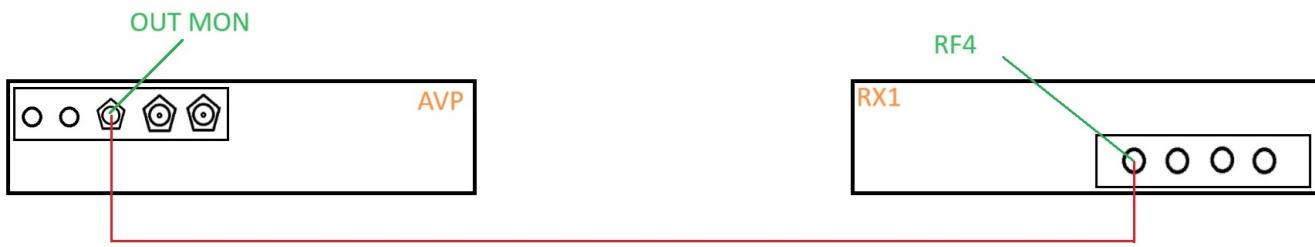
The Monitor F-Type output of the AVP is connected directly to the RF input of the RX1 (RX4 is on the left). There is no up-convertor or attenuator in use.
