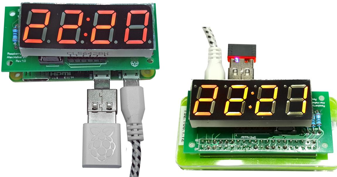
Above we can see the Clock working in 'Normal' mode on the left, and in 'Inverted' mode on the right.
