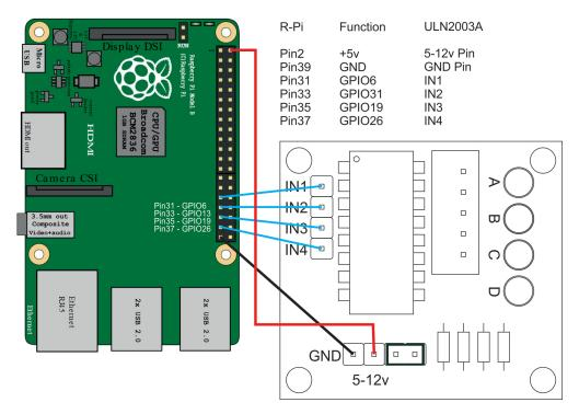
Yep, six wires is all we need. If you are using the same stepper motor as in this example (the 28BYJ-48) then the total current draw of your Pi will be around 500mA (depending on what you have plugged in). This is will within the 1Amp you can get out of the 5V supply.
