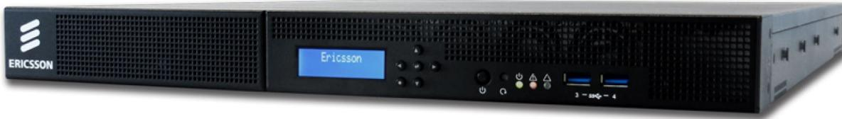
The CE1 is the replacement for the AVP HEVC. It is M1 based like the RX1/MKSP but has some different hardware to allow it to perform encoding. The Main difference is the VEGA (Mellanox) card that can do (at this time) up to 4 HD encodes or 1 x UHD Encode. The CE1 supports HEVC and H264 at resolutions up to 2160p50 4:2:2 10 bit.
